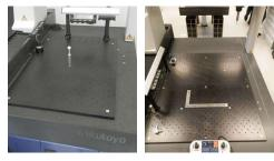
The base plates provide multiple possibilities for fixing fixtures and accessories or even the direct construction of jigs on the CMM.
