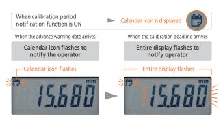
The calibration warning date and calibration due date can be set. A warning is displayed when the calibration time approaches and on the calibration date to prevent skipped calibration. This is an effective function for proper management of the Digimatic gage.
